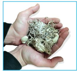
• With the overflow channel blocked, hot glue will drip down inside the body of the machine and form around the electrical components. Over time this will cause damage to the internal components of your edgebander, which will cause the unit to stop functioning. It is your responsibility to maintain your equipment, **FAILURE TO DO SO WILL VOID ITS WARRANTY!**
