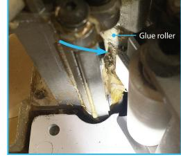
• The pictures above shows a build up of dried glue in the out-feed and work areas this has caused the edgebander roller to become contaminated. This will effect the quality of the finish.
